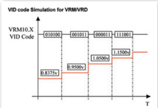
The 62000P Supplies provide 8 output TTL bits with timing control. These control lines can be used for VID control of VRM or to control other discrete signals.
