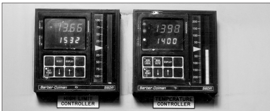
Figure 9-2 - Photo of furnace pyrometer showing metal temperature
