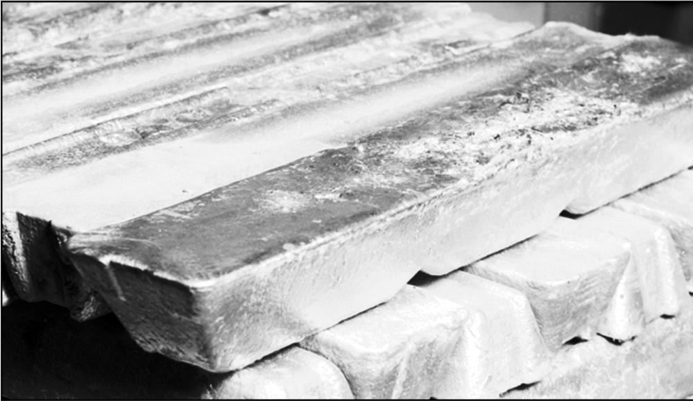
Figure 8-28 - Photo of the top of an ingot showing shrinkage
