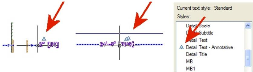
You can view, add, and delete the object scales supported by an object using the Annotation Object Scale dialog box, which is displayed using the OBJECTSCALE command. This command appears on the Annotation Scaling panel on the Annotate ribbon tab. The list of available scales displayed in this dialog box comes from the general AutoCAD Scale List, which you can customize using the SCALELISTEDIT command. This command also appears on the Annotation Scaling panel on the Annotate ribbon bar.
