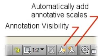
The second tool (the annotative lightning bolt button, which toggles the ANNOAUTOSCALE system variable) enables you to automatically add scales to annotative objects when the annotation scale changes. For example, if the annotations in the current viewport only include an Annotative object scale of 1:50 and you want to change the viewport/annotation scale to
