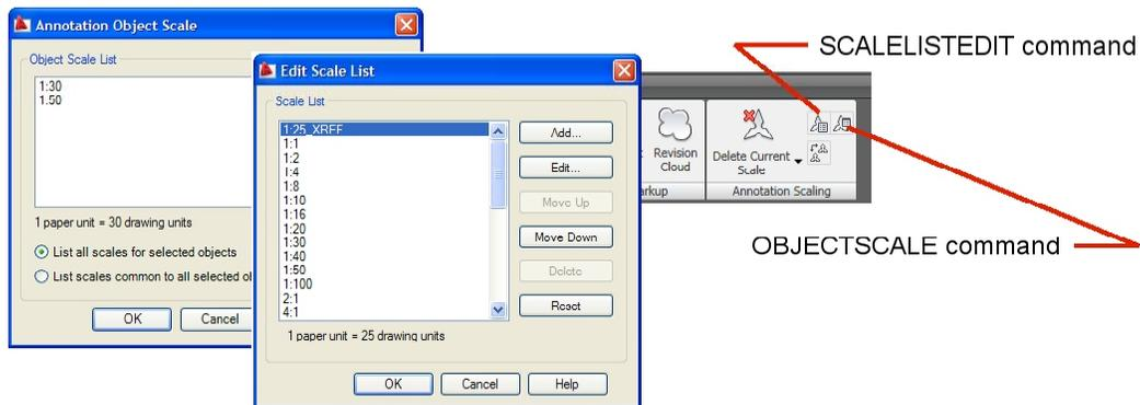
The annotative scales of an object determine the size as well as the visibility of the object's scale representations. When a viewport or the Model tab is set to a particular annotation scale, only the annotative objects that support the current annotation scale are normally displayed.
