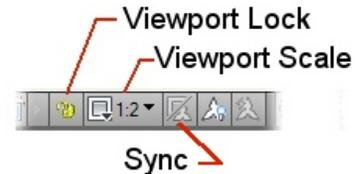
The Viewport Lock is displayed on the Status Bar when a layout viewport is selected or active. You can lock and unlock a viewport using this button or using other methods, including the right-click menu and the Properties or Quick Properties palettes. Locking a viewport after setting an appropriate viewport scale prevents you from inadvertently zooming or changing the scale.
