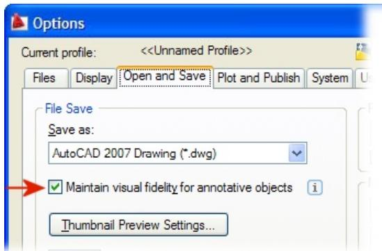
The following steps give an overview for using visual fidelity control to round trip edit drawings that use annotation scaling to early versions of AutoCAD and back:
