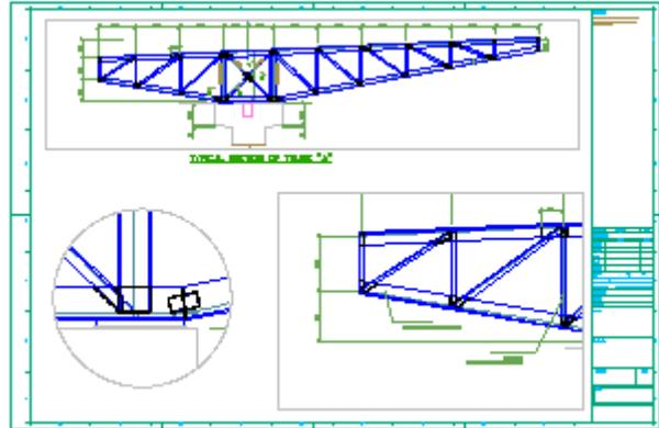
This drawing contains multiple viewports at different scales. The geometry is drawn at full scale, but each view of that geometry is scaled to fit on the sheet of paper. Using a traditional approach, in order to create dimensions that appeared at a uniform size in relation to the overall drawing sheet, you would have to use a different dimension scale factor and draw on a different layer in for each viewport. But annotation scaling eliminates these additional steps.
