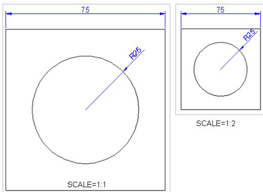
With annotation scaling enabled, AutoCAD automatically calculates and applies properties, such as text height, based on the current annotation scale. It also uses the annotation scale to determine which annotations are visible in which viewports. You can control the location of individual scale representations while having the information itself coming from a single source.
