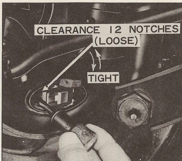
Fig. 7 Front Brake Adjustment
