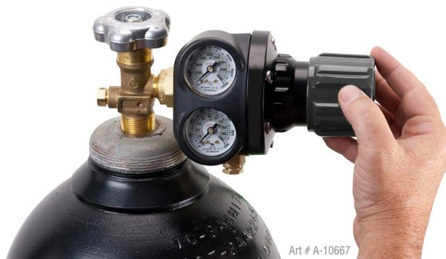
Figure 3-19: Adjust Flow Rate
